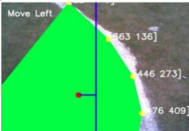
Fig. 5: Polynomial mapped over the detected points
